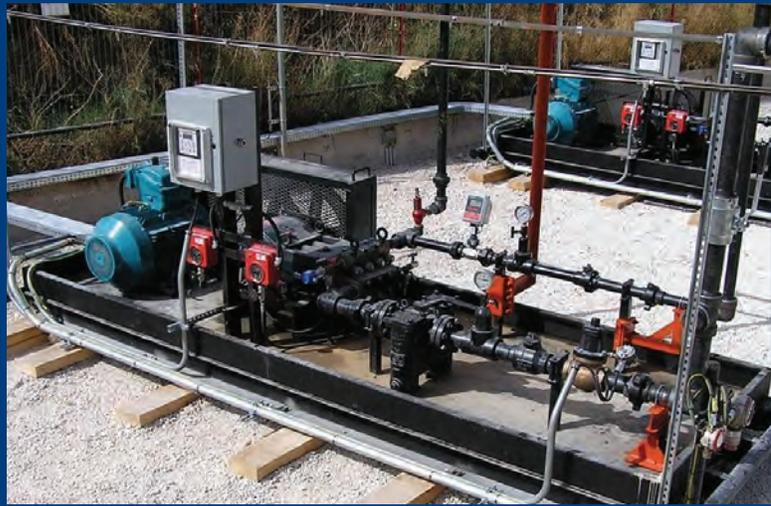
*Jet pump oil extraction process - surface pump supplying high-pressure water to down-hole jet pump*
