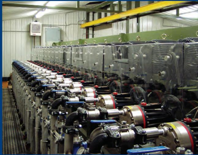
Enhanced oil recovery - pumping shear-sensitive polymers
