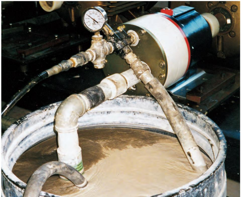
Pumping ceramic slurry at 40% solid content.
